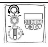
The potentiometer will control the motor shaft rotational speed.
