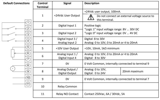
The analog output function may be configured using parameter P-25, which is described in section 6.2 Extended Parameters on page 17. The output has two operating modes, dependent on the parameter selection.
